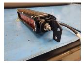
Place the lamps together to make sure you have the proper bracket on the proper side. Be sure the SAE certification is at the bottom left corner of each light.
