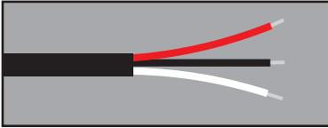
Red Wire (+12V DC) = Forward Projecting Trigger
