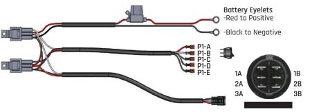
Drill 3/4" Hole to Install Switch
